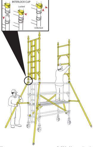
Fit 2 pairs of diagonal braces in opposing directions between the 3rd and 5th rungs and the 5th and 7th rungs.
