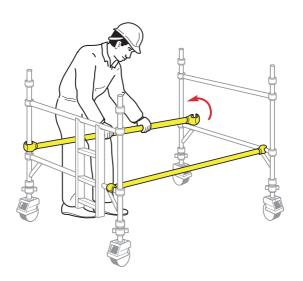
Fit 2 additional end frames, ensuring the frame interlock clips are engaged. Fit 2 diagonal braces (blue) in opposing directions, between the 1st and the 3rd rungs. Ensure the frames are vertical and level by checking with a spirit level and setting the adjustable legs as required.
