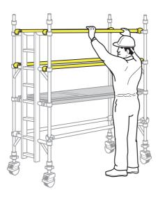
Fit 2 diagonal braces in opposing directions between the 1st and 3rd rungs. Ensure that the frames are vertical and level by checking with a spirit level and setting the adjustable legs as necessary. Fit stabilisers (see notes on page 30). Fit the next pair of end frames and check the frame interlock clips are engaged.
