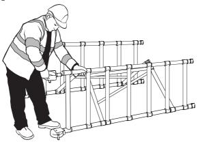
When using adjustable legs for uneven or sloping ground, push 4 castors into 4 adjustable legs and then insert the adjustable legs into the bottom of the base unit. The bottom of the base unit may be identified by the bottom end casting – see diagram.
