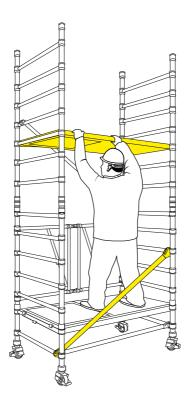
4 Climb the tower on the inside using the rungs of the end frames. From the protected trapdoor position, fit 4 horizontal braces as guardrails, 2 and 4 rungs above the platform (the 12th and 14th rungs of the tower) on both sides of the tower.
