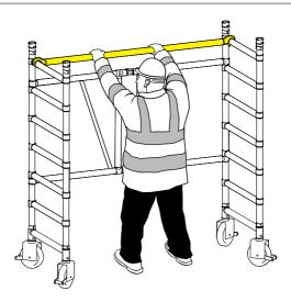
3 Fit a horizontal brace (red) as a guardrail on the top (7th) rung, on the hinged frame side of base unit.
