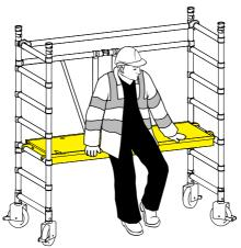
5 Climb onto the platform in the sequence shown From the seated position, fit horizontal braces as guardrails on the 5th and 7th rungs on the open side of the base unit. Do not stand on the platform until the guardrails are in place.
