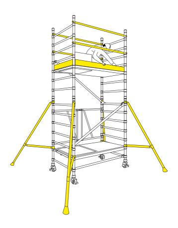
IMPORTANT. Always ensure braces are fully locked in position.
