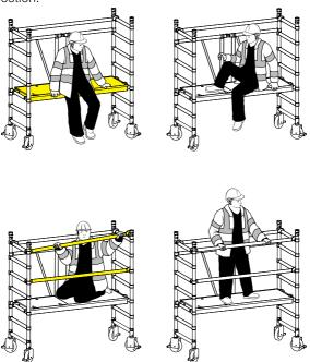
6 If your risk assessment shows it is necessary, fit a set of toeboards to the platform. Check there are no gaps through which any materials could fall and that the trapdoor opens correctly. The tower is now complete.
