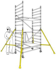
6 Climb the tower on the inside using the rungs of the end frame. From the protected trapdoor position, fit 4 horizontal braces as guardrails, 2 and 4 rungs above the platform (the 12th and 14th rungs of the tower) on both sides of the tower.
