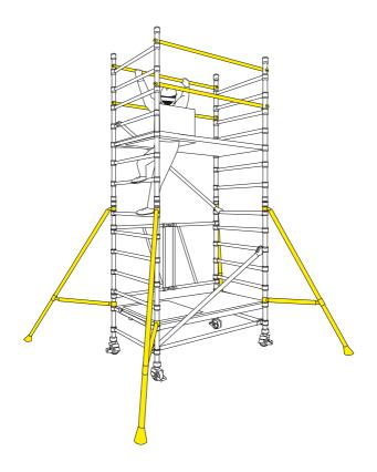
5 Fit a 4 rung guardrail frame to each end of the tower. Ensure the frame interlock clips are engaged.
