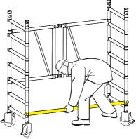
3 Position a temporary platform on the 2nd rungs of the tower. Engage the wind locks, underneath the rungs, at both ends of the platform.
