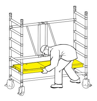
3 Fit a 7 rung lift frame to each end of the base unit. Ensure the 4 frame interlock clips are engaged.
